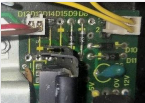
Rectifier diodes - some are missing on this photo
