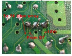
The right pin on this picture is the 12V, but in the original way the 2N3904 is mounted, the 12V is connected to the emitter of the 2N3904: that is definitely wrong.
