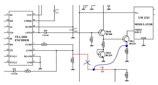
Lift the capacitor on the side where the cross is.
