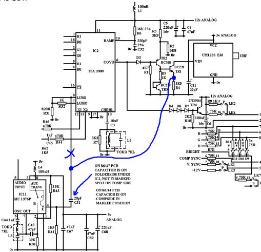
As the text at the blue arrow sais, this capacitor is on some models on the component side in the position that shows C31, but with other models it's on the bottom – if I remember correctly it's under the TEA2000 then.
